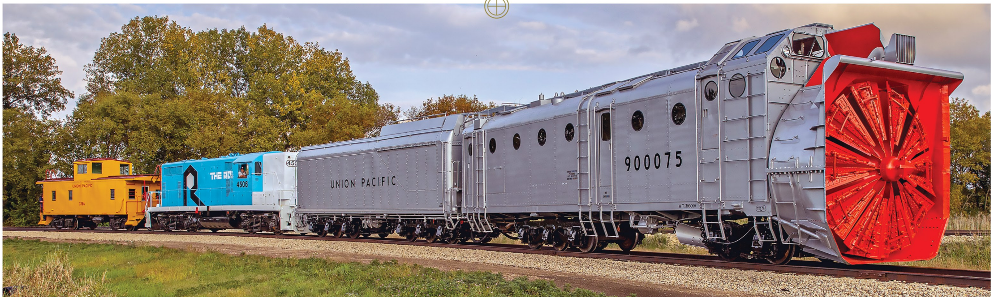
Freshly painted Union Pacific rotary snowplow & tender 900075 (built by Lima in 1949) is powered by Rock Island 4506, an Electro-Motive Division GP-7R locomotive (1952) pulling Union Pacific caboose 3786 (1942). The distinctive 1970's era paint scheme on The Rock EMD locomotive commemorates 100 years since the 1922 establishment of one of the nation's most successful locomotive builders. Photo by Rob Schreiner.
