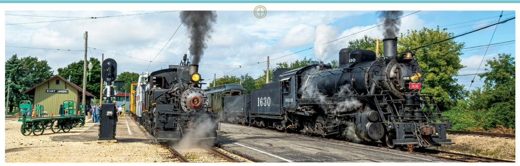
J. Neils Lumber Co. No. 5, a three-truck Shay geared locomotive built by Lima in 1929, and St. Louis - San Francisco (Frisco) No. 1630, a 2-10-0 Decapod (Baldwin, 1918), are steamed up and prepared for service. Shay No. 5 operated in the Pacific Northwest logging industry and was the first steam locomotive to operate at IRM in 1966. Decapod No. 1630 was built for export to Russia but remained in service in the U.S. until it came to IRM, where it has operated since 1972. Photo by David Zeman.
